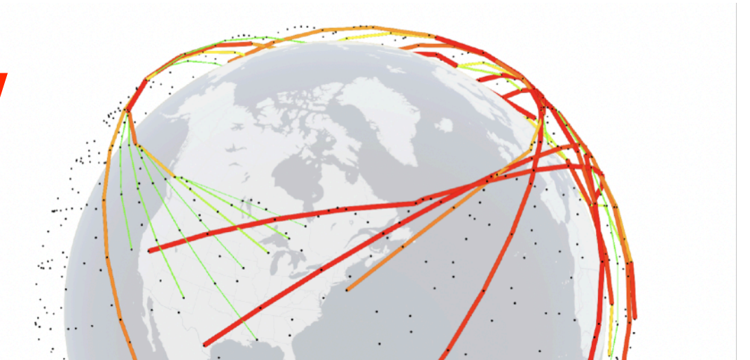
Fig. 15: Constellation-wide utilization. On Kuiper, the transatlantic paths are highly congested for our tested traffic matrix. The red / thick ISLs are heavily utilized, while green / thin ISLs have minimal traffic. ISLs with no traffic are excluded.
